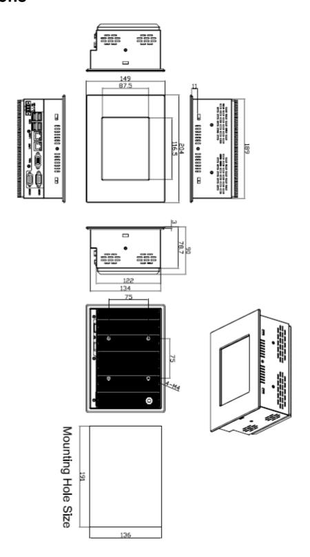
Figure 1.1: Dimensions of EX-96057A
