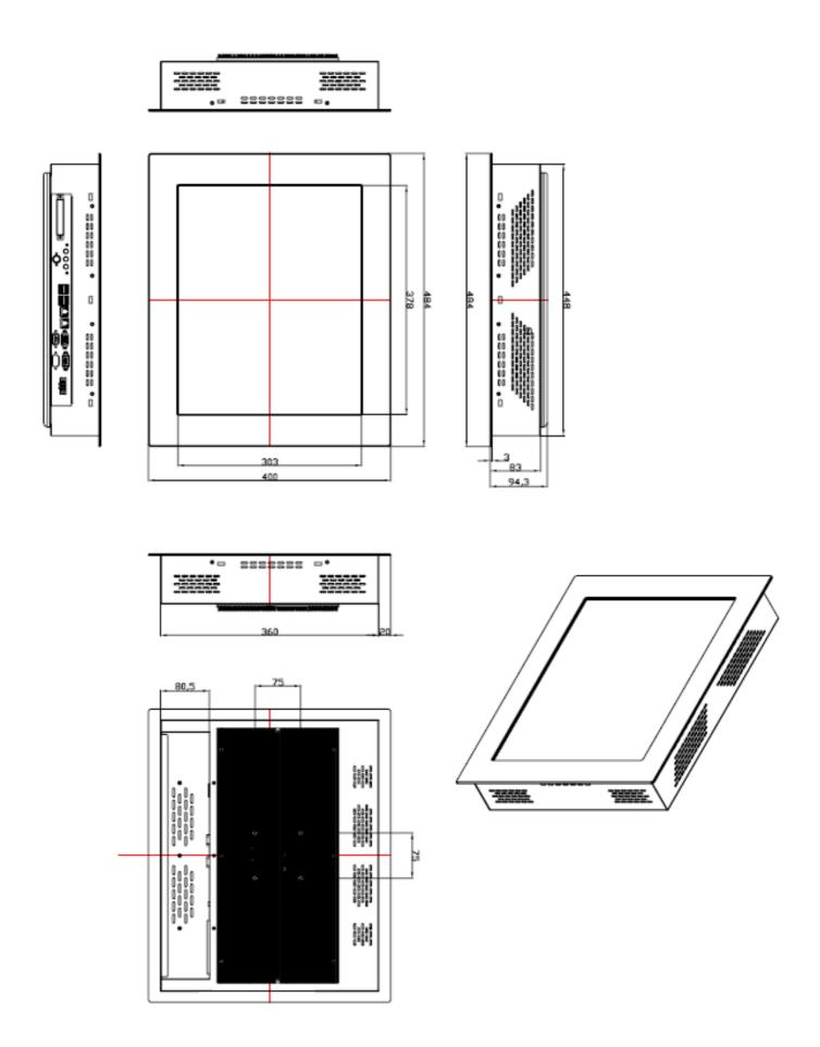
Figure 1.7: Dimensions of the EX-96197A
