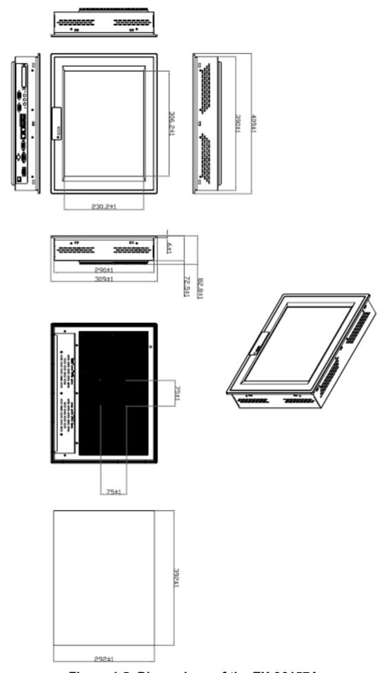
Figure 1.5: Dimensions of the EX-96157A
