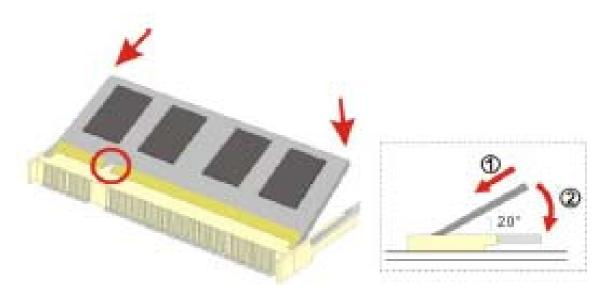
Figure 2.2: Installation of Memory Module
