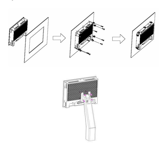
Figure 1.10 Panel mounting and VESA mounting of the EX-96XX7A
