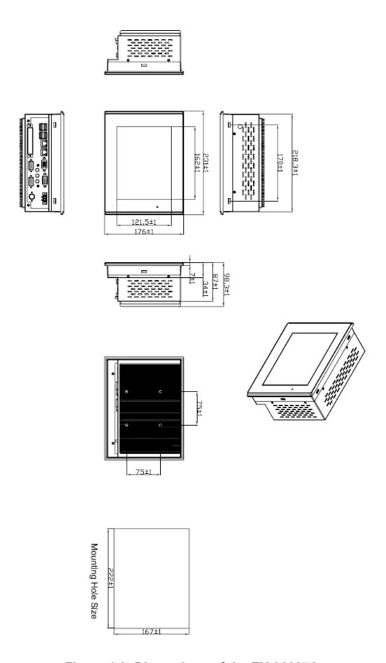
Figure 1.2: Dimensions of the EX-96087A
