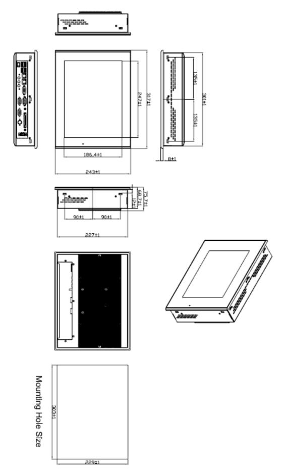
Figure 1.4: Dimensions of the EX-96127A
