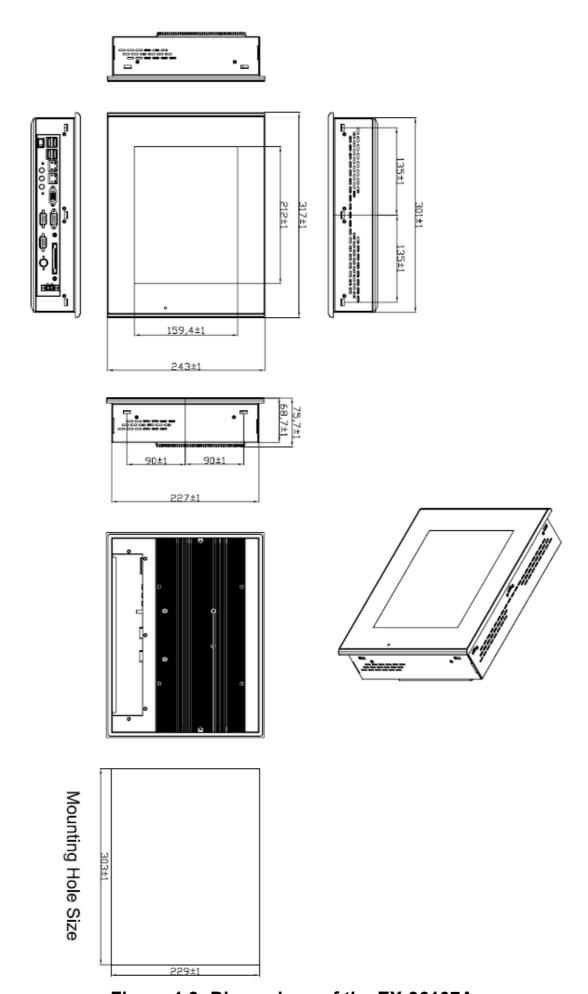
Figure 1.3: Dimensions of the EX-96107A
