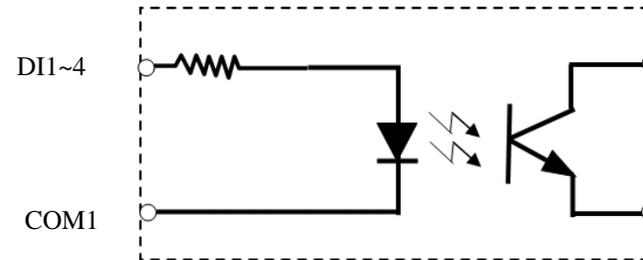
DIx: Isolated digital input channels
