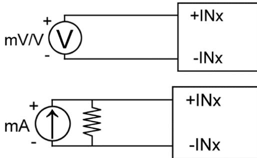
**EX9017P** Analog I/P Channel 6 and 7 wire connection, while the jumper JP1 setting is 8 differential mode.
