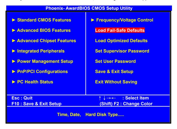
Pressing Y loads the BIOS default values for the most stable, minimal system. Performance.
