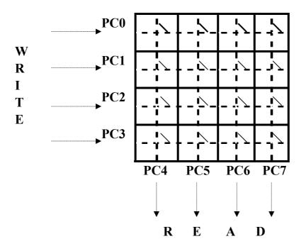
Install the corresponding RP(s) to pull high the digital input lines. Configure Group #1 Port C-upper as read port and Port C-lower as write port. In a loop, send below patterns to Group #1 Port C:
