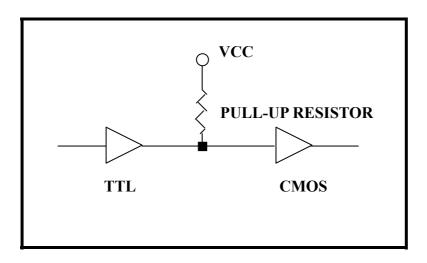
**Digital Input for Open/Short Switch Detection** – A pull-up resistor must be connected, especially at long distance wiring, to ensure logic high input level.
